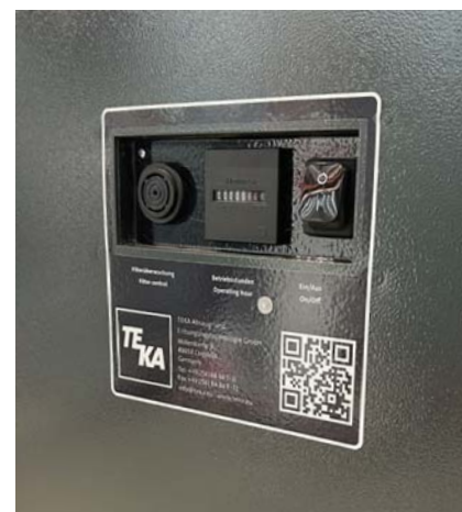
Clear controls with operating hours counter and signal horn
