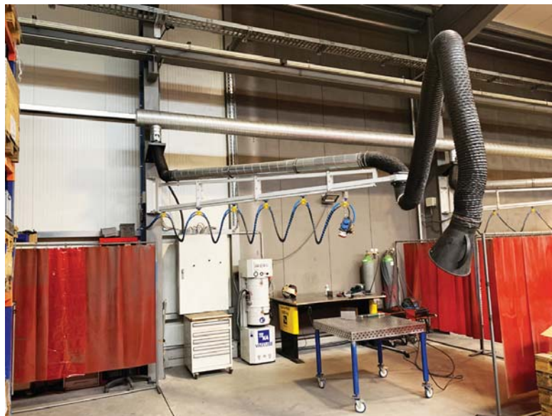
Suction arm with wall bracket and guide rail
