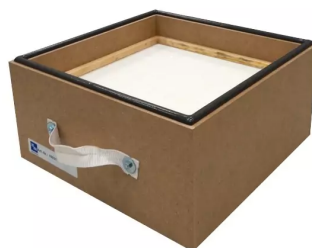
HEPA filter H14, 592x592x300 mm, ViroLine Tower Product No.: 20170260114
