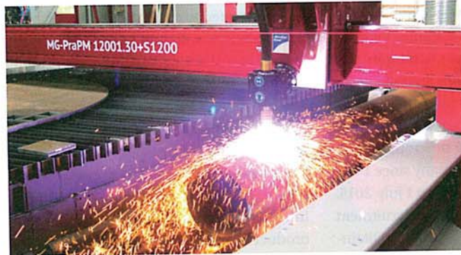
The 3D tube and profile machining rates among the wide range of tasks of the multifunctional cutting unit.
